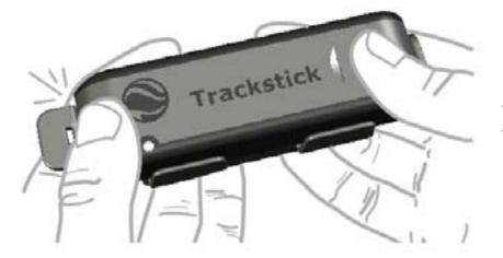
Mounting Trackstick into the belt clip or magnetic mount Position a notch at either end of the clip into a groove at one end of the Trackstick and squeeze the Trackstick into position at the opposite end until the second notch snaps into place.
