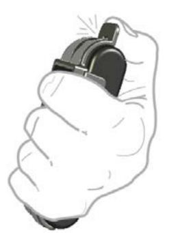
Removing the belt clip or magnetic mount Grip the Trackstick firmly in one hand and with your thumb push the tab at the top like you would click a pen. This may require some amount of pressure, but the clip will detach with a little force.
